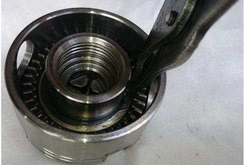
A close-up view of the chuck with external circlip pliers being used to remove the retaining ring from the outer edge.        |
