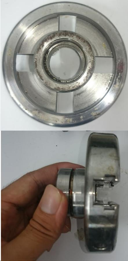
The top image shows the inner surface of a metal chuck body with a scroll ring. The bottom image shows a hand holding a metal jaw slide, which is a semi-circular component with a central hole and a dimple. |
