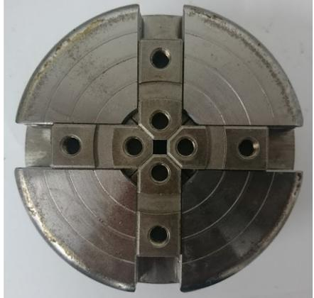
The image shows the fully reassembled chuck, which is a circular metal component with four jaw slides inserted into its slots. The jaw slides are numbered sequentially in a clockwise direction.            |
