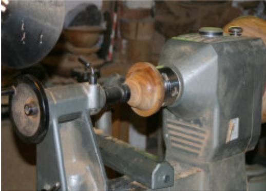
10. Take a small solid block, preferably flat on both sides, and using your lathes tailstock, compress the block up against the workpiece.
