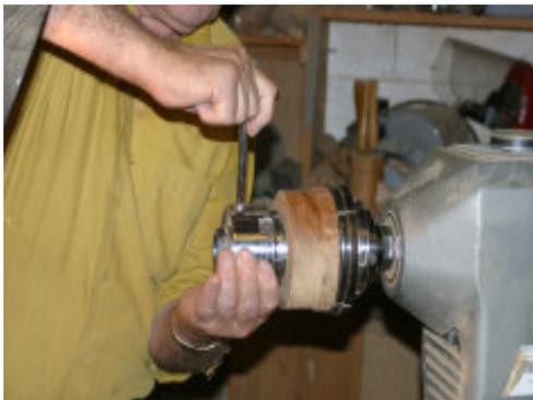
7. The 50mm Jaws will now lock in and secure the wooden work piece.
