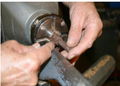
22. Part off the legs using a parting tool.
