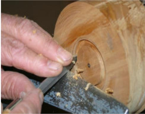
5. There are different ways to turn the bowl. In this project, Bill used the parting blade to form the groove in the bowl. To remove the remaining material a bowl gouge was used to face off the excess wooden stock.
