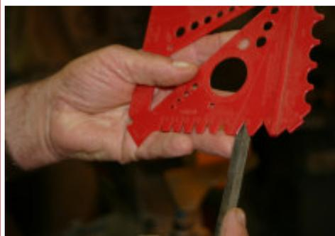
3. For quick grooves in the bowl use the Angle Checker function on the gauge and check the angle of the parting blade.
