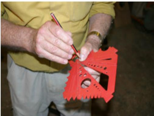
16. Using whatever scrap wood you have to make dowels (a light, clean & hard white wood is good for this) mark the centre on your stock piece for your desired dowel using the centre finder.
