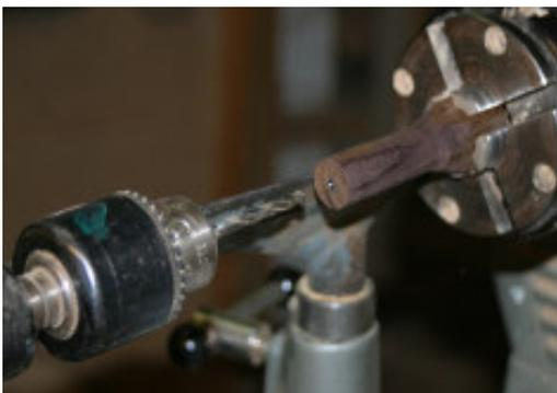
21. Once the legs are turned, drill the legs to your preferred depth, using a drill bit the same size as your dowel.
