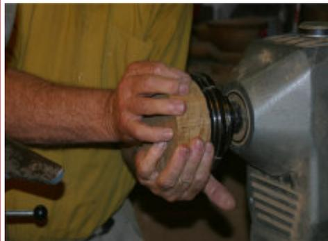
1. Using a Woodworkm Screw, a blank is attached to a NOVA G3 chuck.
