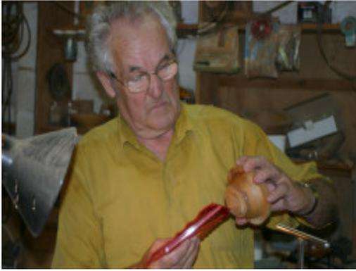
14. Disengage the workpiece from the 50mm jaws and turn the piece over. Engage the glue block end to the 50mm jaws.
