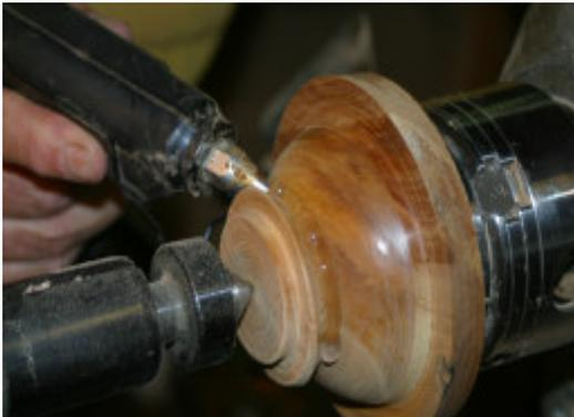
11. Using a hot glue gun, apply the glue and connect the block to the workpiece. For safety reasons ensure that the circumference of both the glue block and the workpiece have sufficient contact glue.
