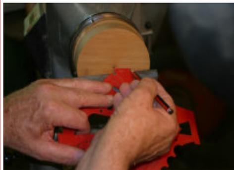
2. The centre of the bowl is found easily using the NOVA 10 in 1 Gauge. The bowl blank is turned completely clean without a spigot.
