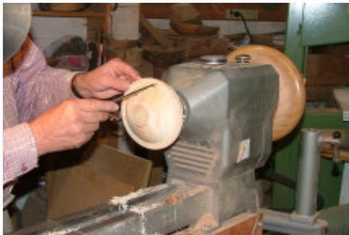
25. Using a protractor function on the NOVA workshop gauge, mark the bowls in 3 separate intervals, 120 degrees each.
