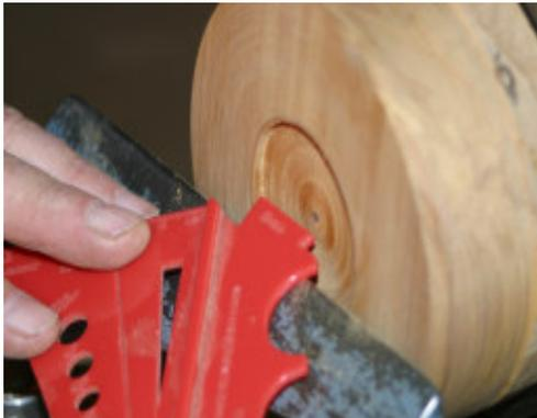
6. Using the Dovetail Function in the gauge, check the recess of the bowl.
