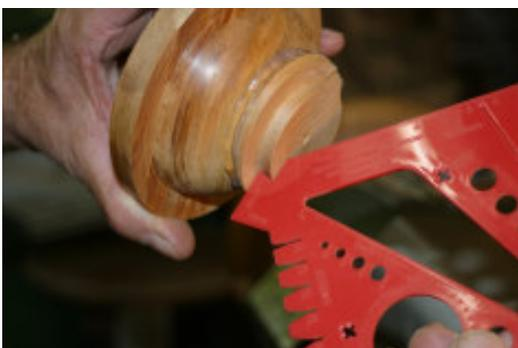
13. Take the NOVA 10 in 1 Workshop Gauge and check the external diameter of the workpiece.
