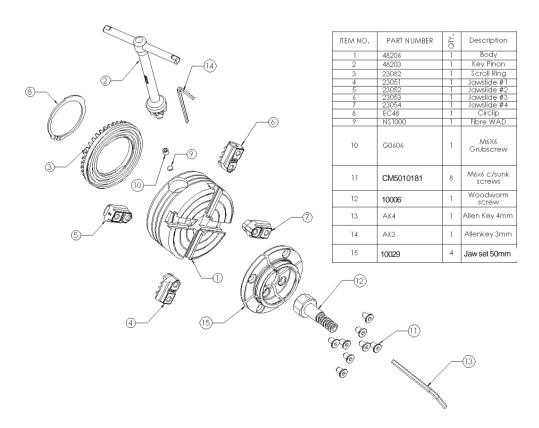
NB: Direct threaded chucks #9 & #10 not used (with the exception of the 4-threaded direct chuck)
