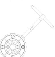
effort. Moving in a clockwise direction will expand the jaws outwards (expansion), and moving the key in an anti-clockwise direction will contract the jaws inwards (contraction). For example, move the handle in an anti-clockwise direction to move the jaws to clamp a work piece inside the jaws, and then move the handle in a clockwise direction to release the work.
