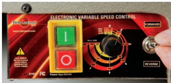
**Master controls on the Comet II include a sealed On/Off switch, the electronic variable speed dial with illustrated speed ranges and a forward/reverse toggle for switching the motor's spin direction.**
