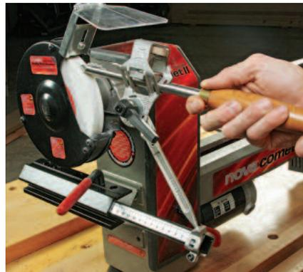
*Swiveling the Versaturn Coupler (top) locks or unlocks accessories, such as the Grinding Wheel (left). Teknatool's Finger Jig (right) can be installed below the grinder for sharpening curved-edge turning tools.*
