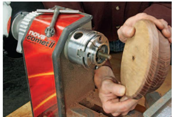
*Another accessory to consider is the NOVA G3 four-jawed scroll chuck, sized especially for the Comet II. It comes with a screw chuck insert and an auto-locking feature that keeps it secured when sanding in reverse.*
