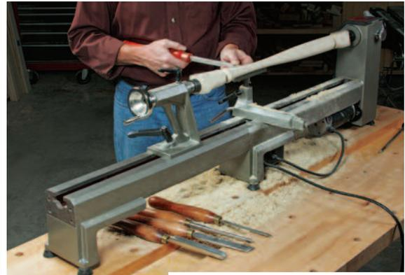
*A bed extension accessory (top) can stretch this midi-lathe's "reach" to full-size lathe capacity. Its spindle has 12-stop indexing (right) for stepping off 30-degree increments on your turnings.*
