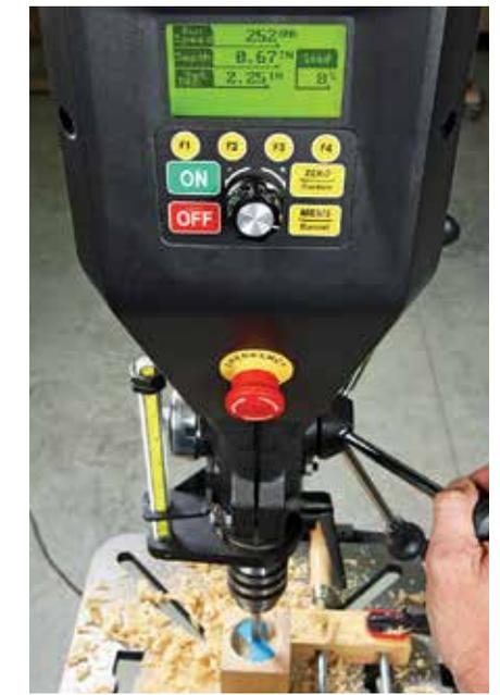
*Want to drill a hole that's exactly 4.388" deep, or any depth up to 6"? Tell the computer those parameters, and Voyager will beep to alert you when you reach it, then turn off automatically.*
