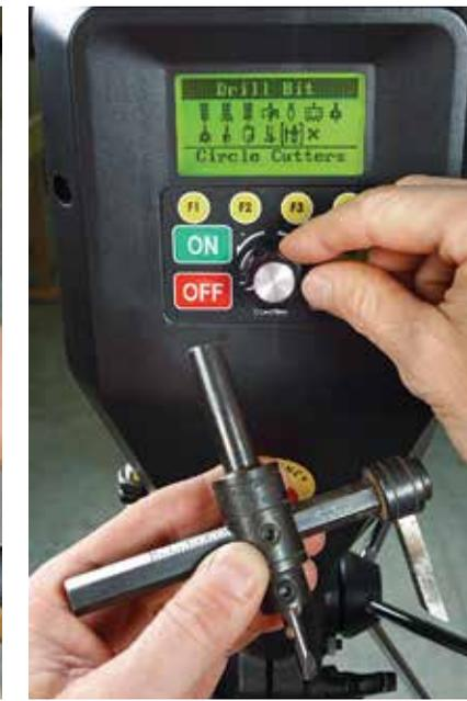
*Uncertain of the correct speed for a task? Just select the bit or cutter style, its diameter and the material type you're drilling into. The drill press will determine the optimal speed instantly.*
