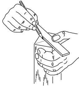
For hardwoods - drill centers and saw diagonals for spur center
