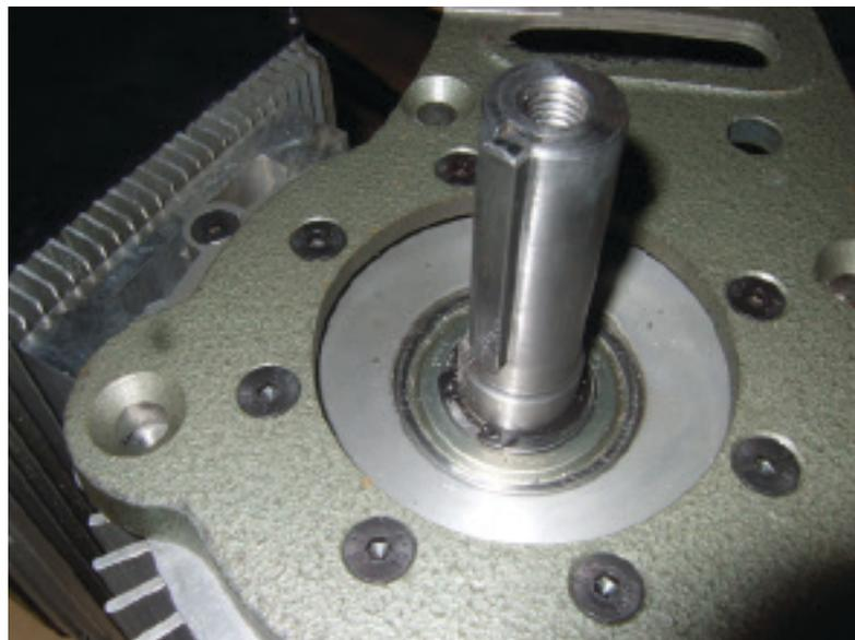
12. Place the motor pulley onto the DVR Package Drive and secure it into place by using the 4mm allen key to lock in the set screw. NOTE: A rubber mallet may be needed to lightly tap the pulley onto the spindle.
