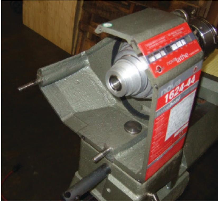
7. Using the 4mm allen key, now remove the pulley from the motor. Also remove the key in the keyway. NOTE: This may require 2 standard screw drivers to gently pry off the pulley. Use at opposite sides underneath the pulley.
