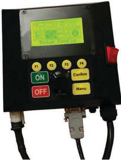
Fig. 7.1: Motor Configuration item highlighted
