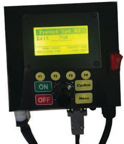
Fig. 2.6: Editing preset speed of 750 rpm
