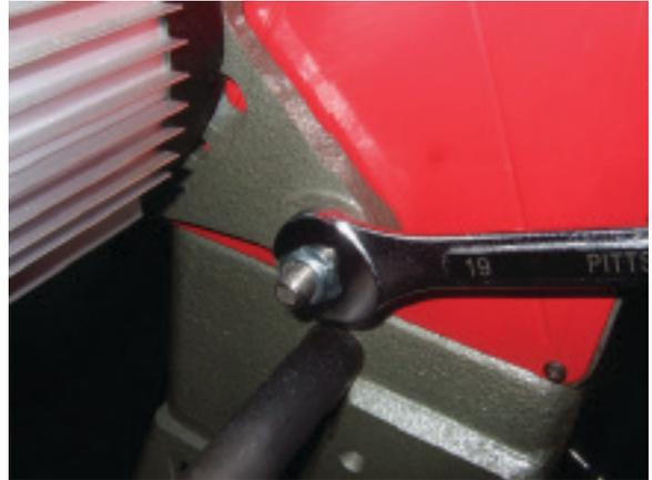
Now remove the cam from the rear motor mount
