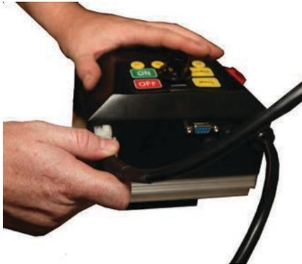
Fig. 1.2: Connecting Molex Connector
