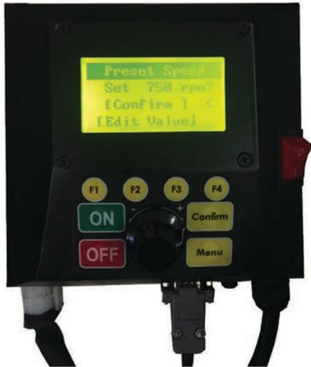
Fig. 2.5: Confirming 750 rpm speed setting
