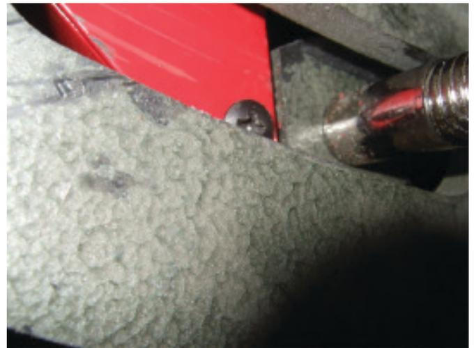
5. With the 6 screws removed you can now go ahead and remove the red cover from the lathe.
