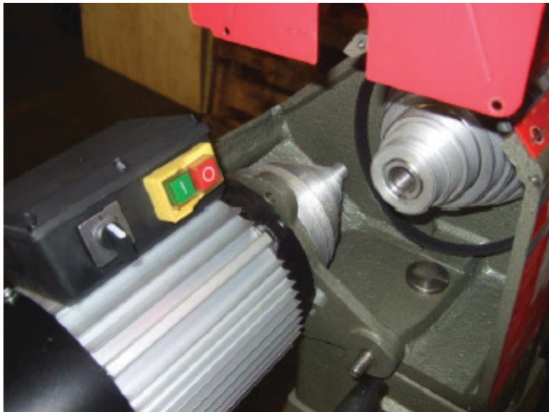
6. With the red cover removed you are now able to remove the old AC motor from the lathe. Be careful! This can be heavy.
