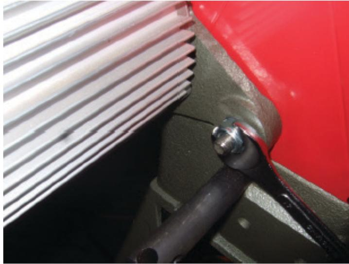
17. With the motor now attached to the lathe, all you need to do now is to place the belt back onto the motor pulley. This is exactly the same process as you would with the standard motor set up. First push the cam up to lift the motor, and then line the belt up on the correct pulley steps, and then release and lock the cam.
