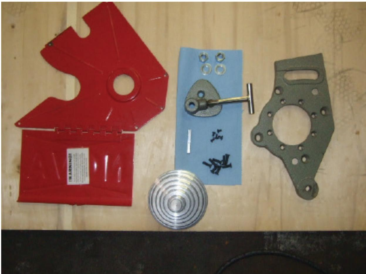
10. You can now start to assemble the DVR Package Drive onto the NOVA 1624-44. The first step is to place the flange onto the DVR Package Drive. **IMPORTANT:** Please not the counter sunk side of the screw holes should be facing upwards. Please line up the flange as shown in the picture, and then using the 4mm allen key, screw in all counter sunk screws.
