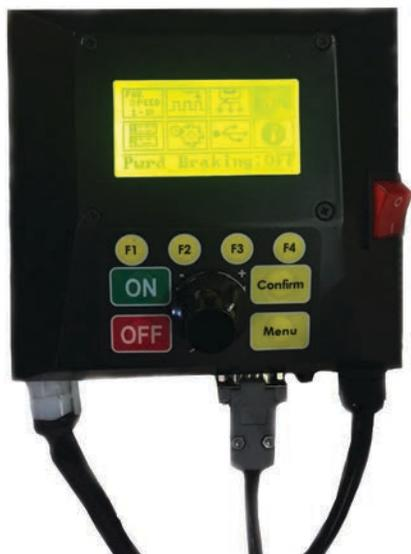
Fig. 5.1: Power Braking highlighted and turned off.
