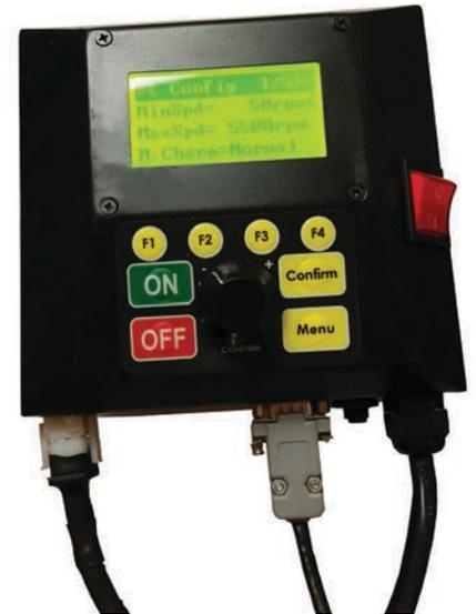
Fig. 7.2: Config 1 - max / min speed
