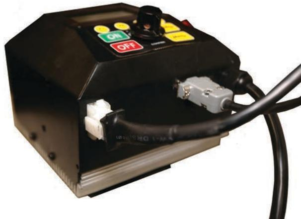
Fig. 1.4: Molex and DB 9 Connector Connected
