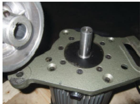
8. With the flange now exposed we will use the 4mm allen key to remove the 8 counter sunk screws that hold the flange to the motor.
