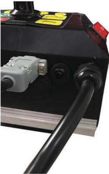
Fig. 10.1: Thermal Reset Switch
