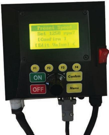
Fig. 2.7: Confirming 1250 rpm speed setting
