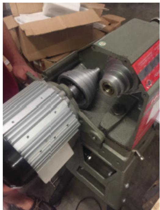
14. Place the cam back onto the rear motor mount.
