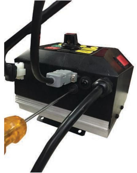
Fig. 10.2: Flicking Thermal Reset Switch back
