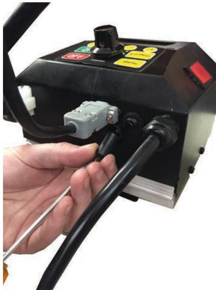
Fig. 10.3: Removing Fuse
