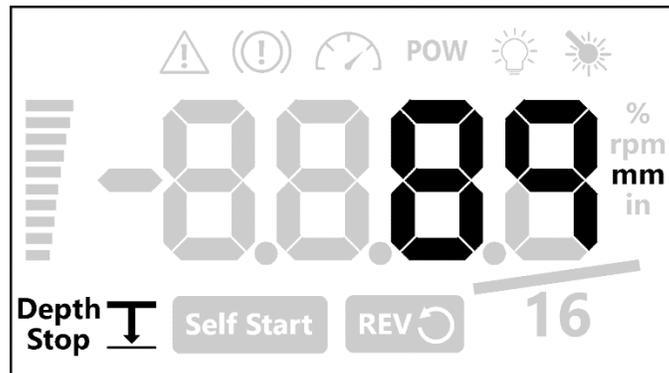
HMI Screen flashes as the displayed depth approaches the set depth
