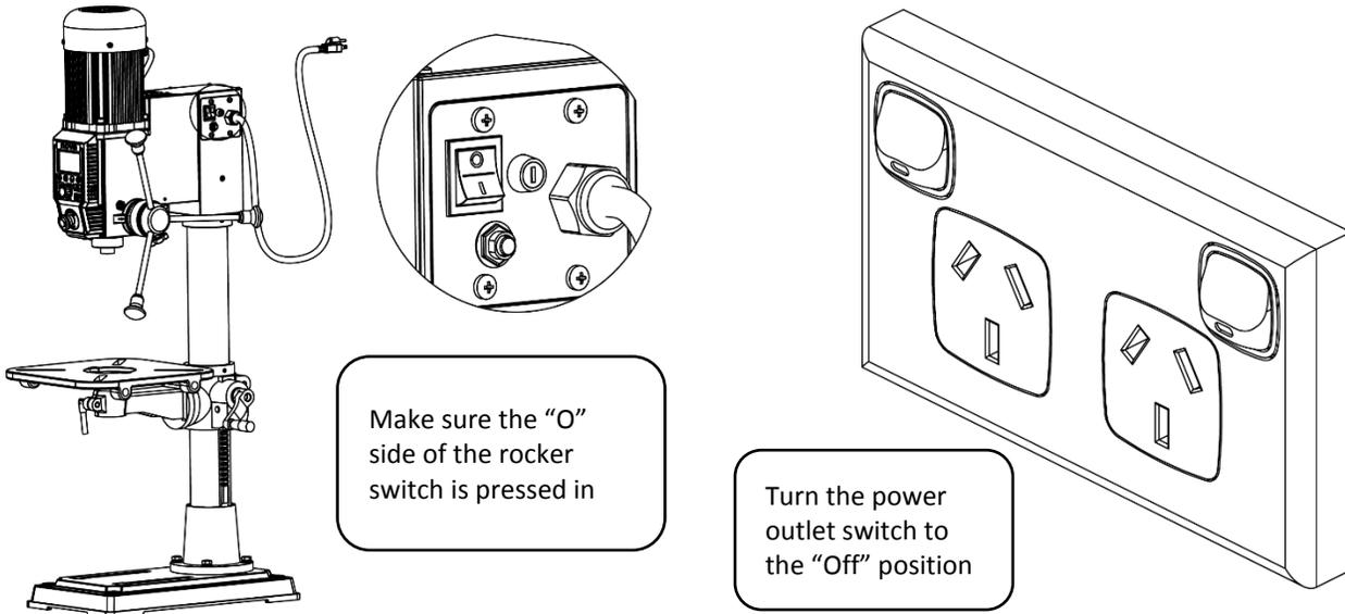
The power cord that is installed on the NOVA Viking drill press will have a three-prong plug which includes a ground prong. The plug must be connected to a matching outlet that is properly installed and grounded in accordance with local electrical codes.
