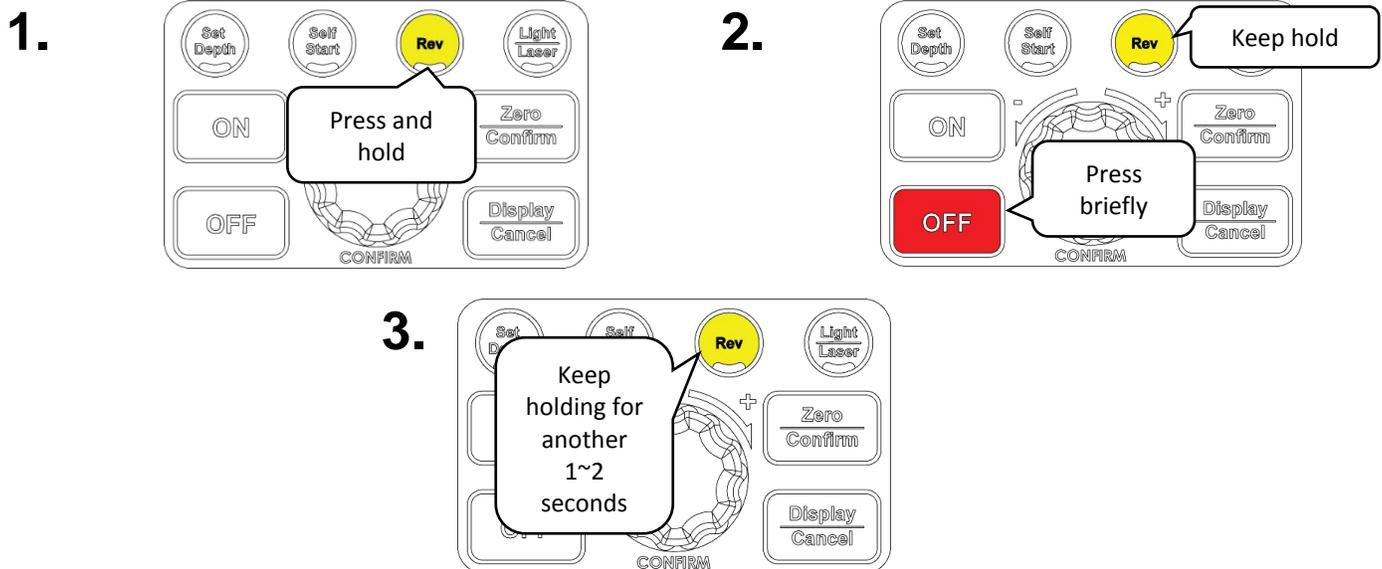
The screen will flash once and a “Sound On” or “Sound Off” message will flow from left to right on the LCD when the command is successfully executed.
