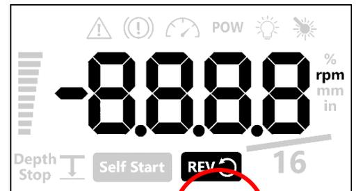
When the drill press is on forward mode, this icon will not be highlighted.
