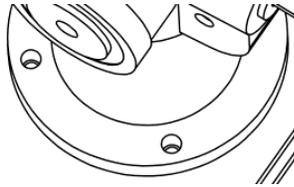
**2** Bolt the bases together with the M10 bolt
