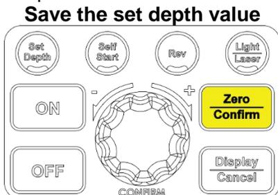
Press the **<Zero/ Confirm>** button once the desired depth is entered on the screen to save the set depth. The depth stop icon will stay lit if the set depth value is saved successfully.
