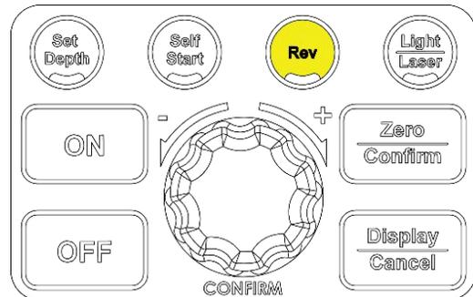
When the drill press is on reversing mode the reverse icon will be highlighted.
