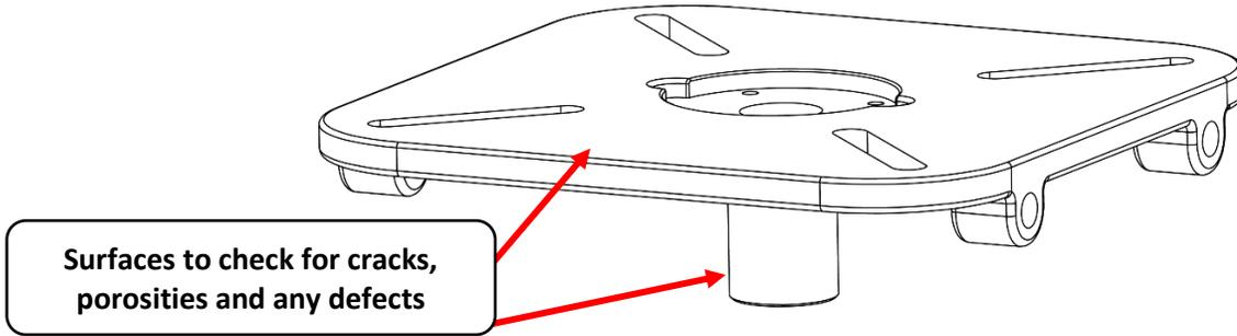
Insert the drill press table into the table arm.
