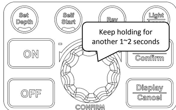
Once the command has been entered successfully, the drill press will begin to display the interface firmware version number and the main control board version number in the respective sequence.
