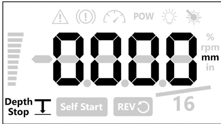
As the drill press readout approaches the set depth, the drill press screen will start to blink and HMI will start to beep.
