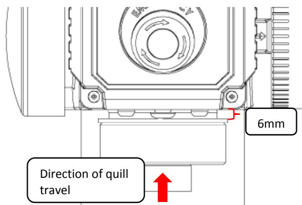
Motor automatically stops with self start function
