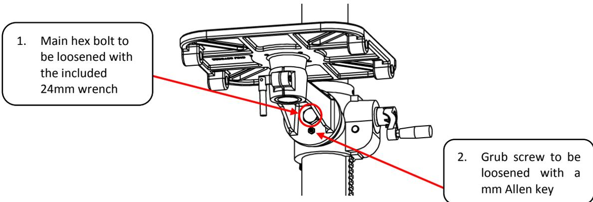
Lock the main table bolt first and then lock the secondary grub screw to secure the table position.
