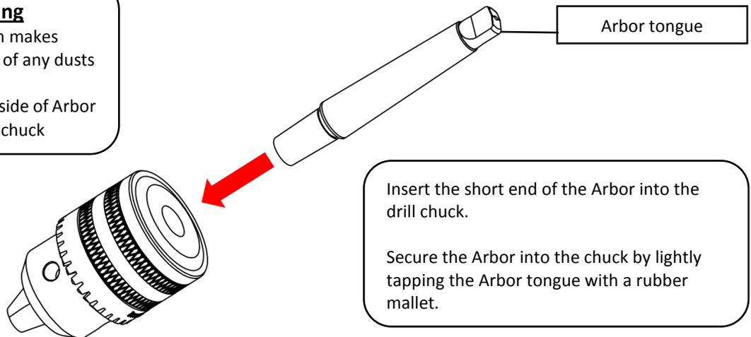
Insert the short end of the Arbor into the drill chuck.
