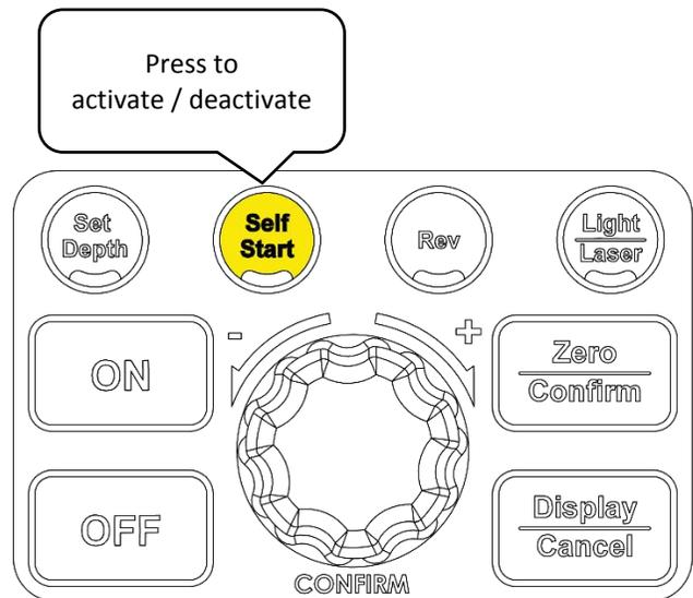
The activation of the self-start function is indicated by the self-start icon on the bottom of the HMI display
