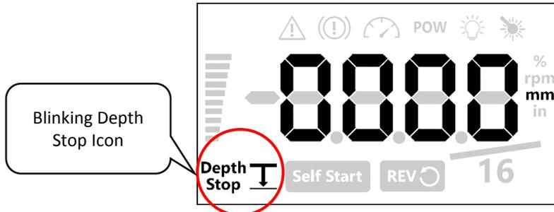
Set the desired depth (measured in the selected units) by turning the speed knob in the clockwise direction to increase the set depth that is displayed on the screen.
