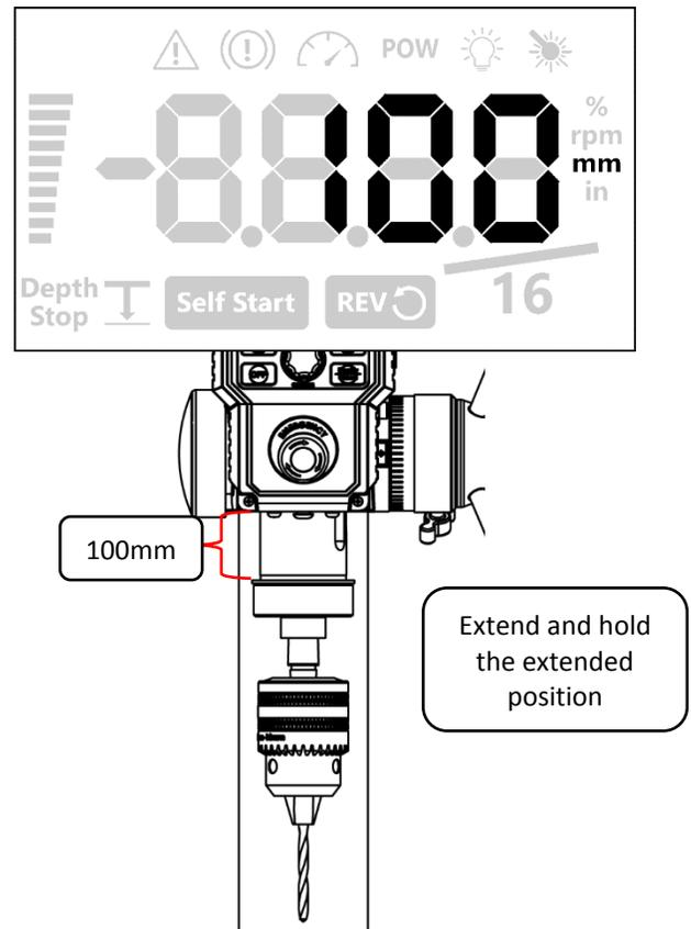
Press and hold the **<Set Depth>** button for 3 seconds while holding the quill in its position. The HMI will beep and it will automatically save the value that is displayed on the HMI screen as the set depth.
