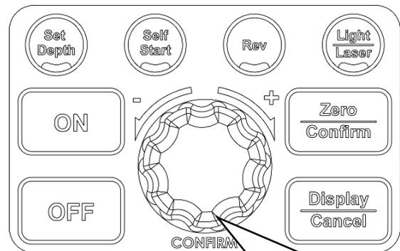
Turn the speed control knob to set the depth on the screen
