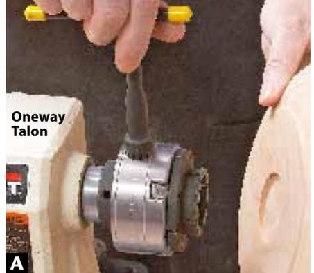
**A** Expanding the jaws inside a recess saves you the effort of later turning away a tenon to finish the project's bottom.
