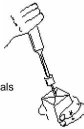
Set spur center with mallet
