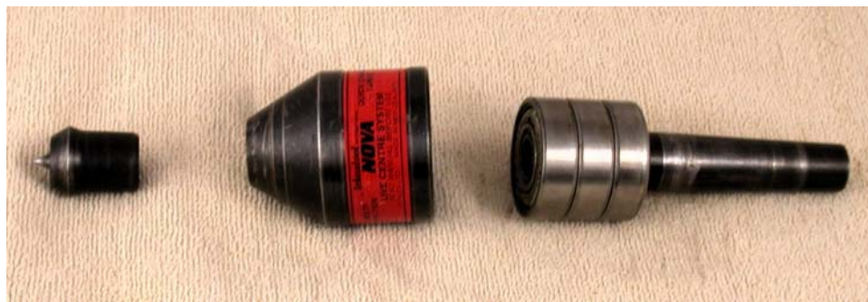
This view shows the Nova Live Center with the rigid external housing removed from the three bearings and the cup center also removed from the housing.
