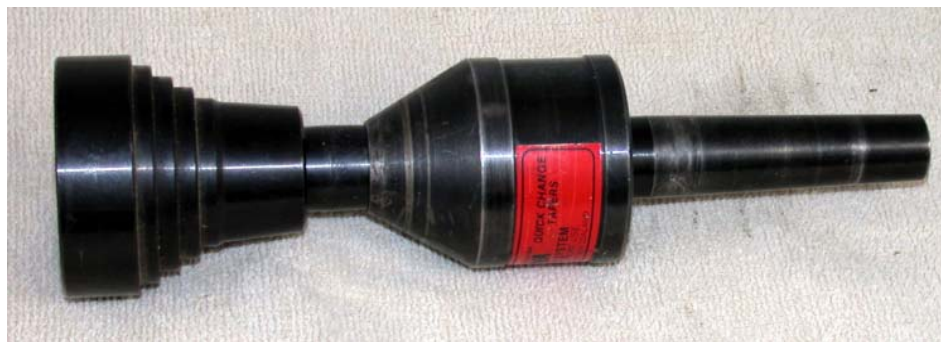
Here the Nova Live Center is shown with the optional cone attached so that it can be used to easily center both square and round stock.
