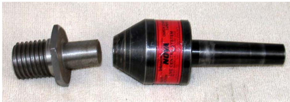
This view shows the Nova Live Center with an optional threaded section to mount a chuck onto the live center. This can be very useful when mounting bowls onto a vacuum chuck.
