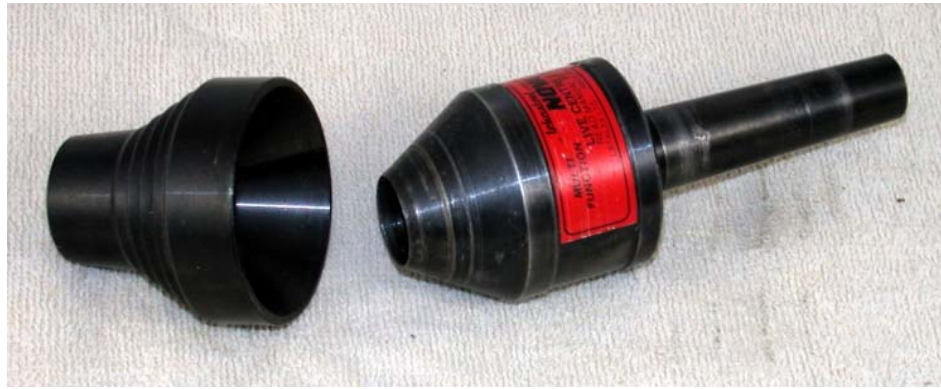
Nova Live Center shown with the optional stepped cone center. The cone center slips onto the tapered nose of the basic live center to provide a number of steps to fit different sizes of holes in the workpiece.
