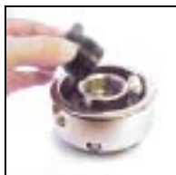
Above Left: Fitting the insert/adaptor to the chuck. Above Right : The Insert/Adaptor fitted.
