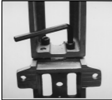
Illustration 3 Joining the Comet Bed and Gap Bed together using M12 cap screws and M10 Allen key.
